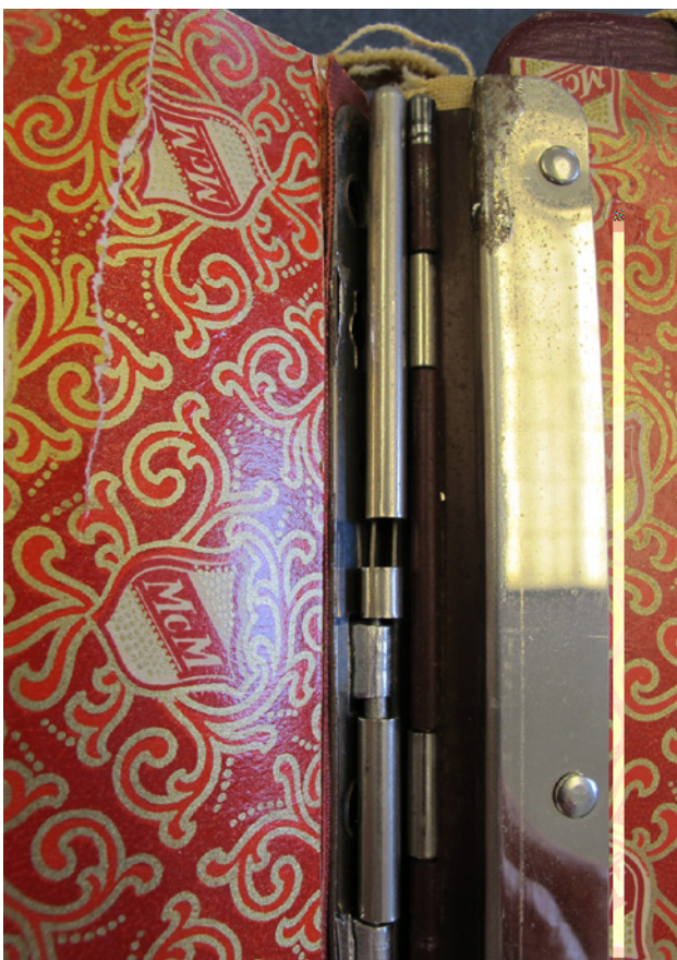
Left: A portion of the mechanism for Appomattox County Deed Book 17, 1916–1917, has rusted and become detached.
