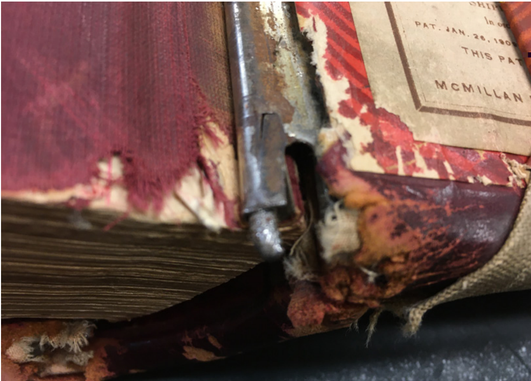
Left: The end of the rod on Dickenson County Chancery Order Book 6, 1921-1926, has broken off, making unlatching it difficult (if not impossible).
